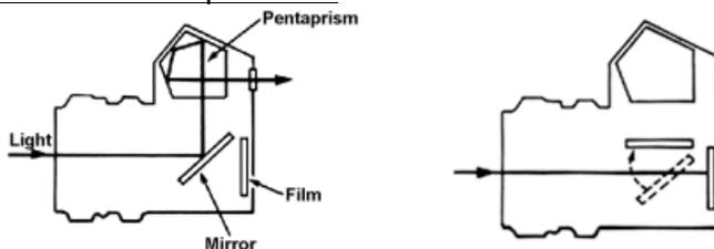
In the SLR camera the light passes through the lens and is reflected off a mirror. The light then passes through a Pentaprism where it is reverted. The mirror remains in the same position until the shutter release button is pressed. When the shutter release button is pressed the viewing mirror rises allowing for the light to pass through to the film plate.
